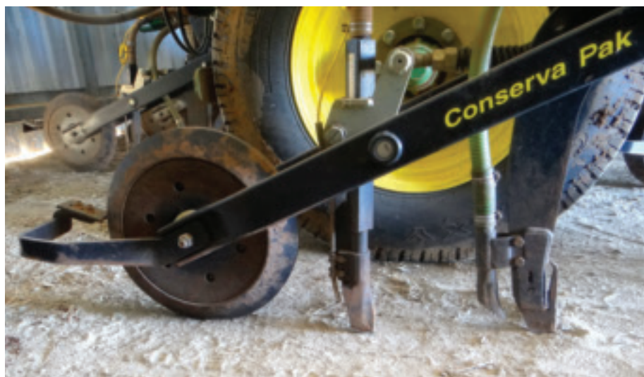
THE CONSERVA PAK IS SET UP TO DEEP BAND GRANULAR FERTILISER AT 100MM, WITH AN OFFSET SOWING TINE, ALIGNED WITH A LIQUID DELIVERY LINE, DEPOSITING SEED AT 25MM.
